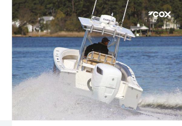
224kW (300hp) gasoline outboard: 98 L/h (26 USG/h)
